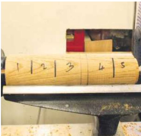
▲ Pic.4 A ratio of \frac{2}{3} ths to \frac{3}{4} ths is about the right proportion for this box. Getting this right can be trial and error, but the more experienced you become the easier this will be
